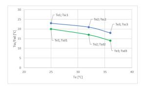
If the unit is controlled according to ambient temperature and its effect on the heating or cooling curve is enabled, the unit changes the water temperature setpoint in either heating or cooling mode at fixed time intervals, based on the difference between the external air temperature measured and the relevant setpoint. The resulting difference is then subtracted from the water temperature setpoint that has been calculated according to the climate curve.
