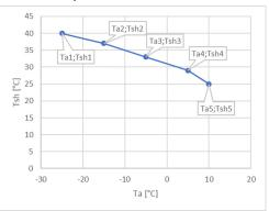
If the unit is controlled according to ambient temperature and its effect on the heating curve is enabled, the unit will change the water temperature setpoint in heating mode at fixed time intervals, based on the difference between the external air temperature measured and the relevant setpoint. The resulting difference is then subtracted from the water temperature setpoint that has been calculated according to the climate curve.
